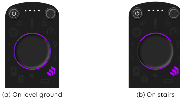
Figure 49. Stair mode display on control panel
