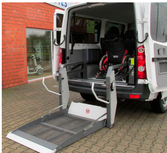
(a) Lifting platform
