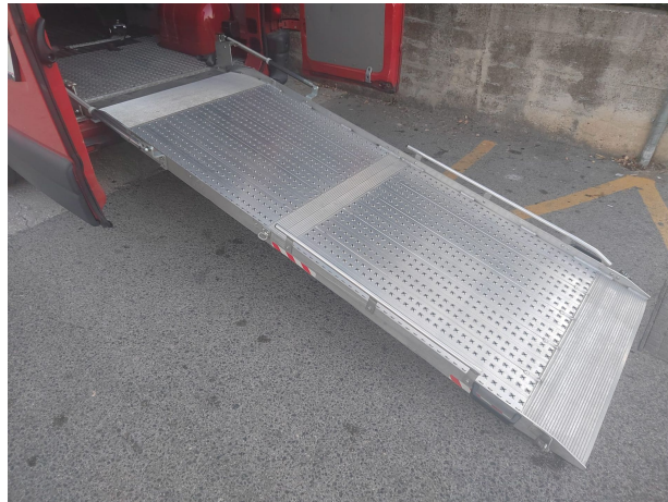
Figure 69. Hazardous, steep folding ramp with threshold at the top
