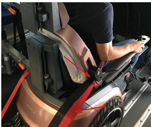
Figure 71. Correct routing of the pelvic belt (red) and 3-point belt restraint (black) to secure the occupant
